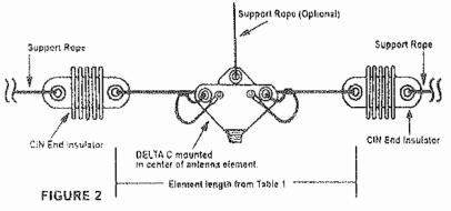
When using the DELTA-C for high power transmitting it may be necessary to remove the SEP Cartridge when VSWR exceeds 2:1.
