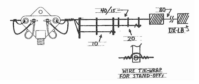
Models DX-CC, DX-DD and DX-EE employ Model SEP gas tube static discharge modules for added safety. They are not used in models DX-LB and LB Plus, since these antennas are used with wide range tuners that have wide SWR voltage swings which could "false trigger" the Model SEP.
