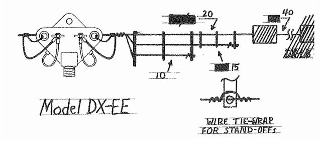
support. The 10 meter wire is run through the bottom holes of the 3 long stand-offs. The end of the 10 meter wire should be run through, and around the last long stand-off and twisted back on itself (about 2 inches) for support.
